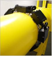
IP 68 enclosure boxes affixed to strap, interconnected for 360° measurement monitoring
