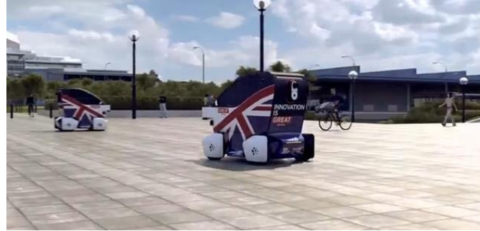
LUTZ, an autonomous pod for two passengers trialled in Milton Keynes
